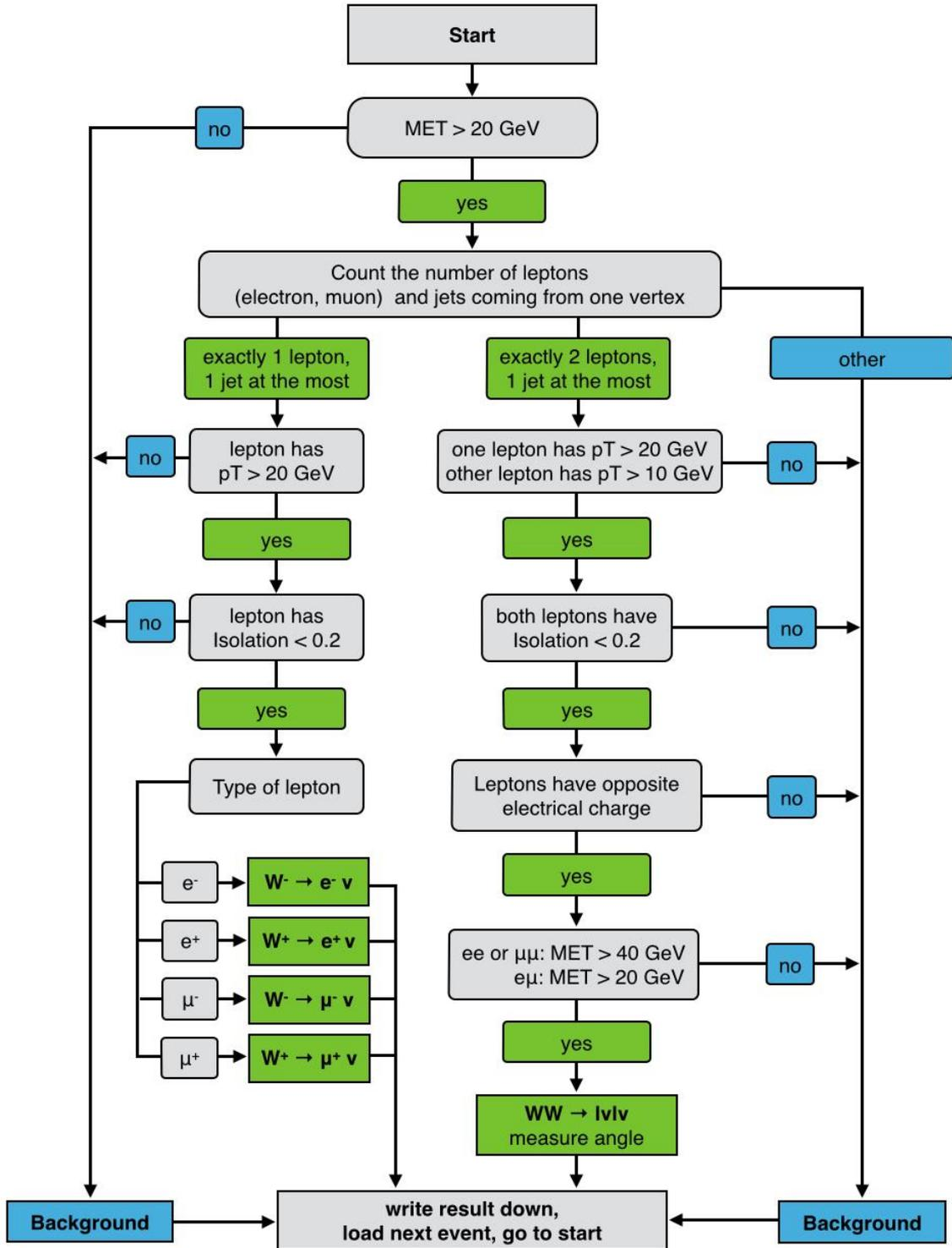
Figure 4: Flowchart for analysis in the ATLAS W path
