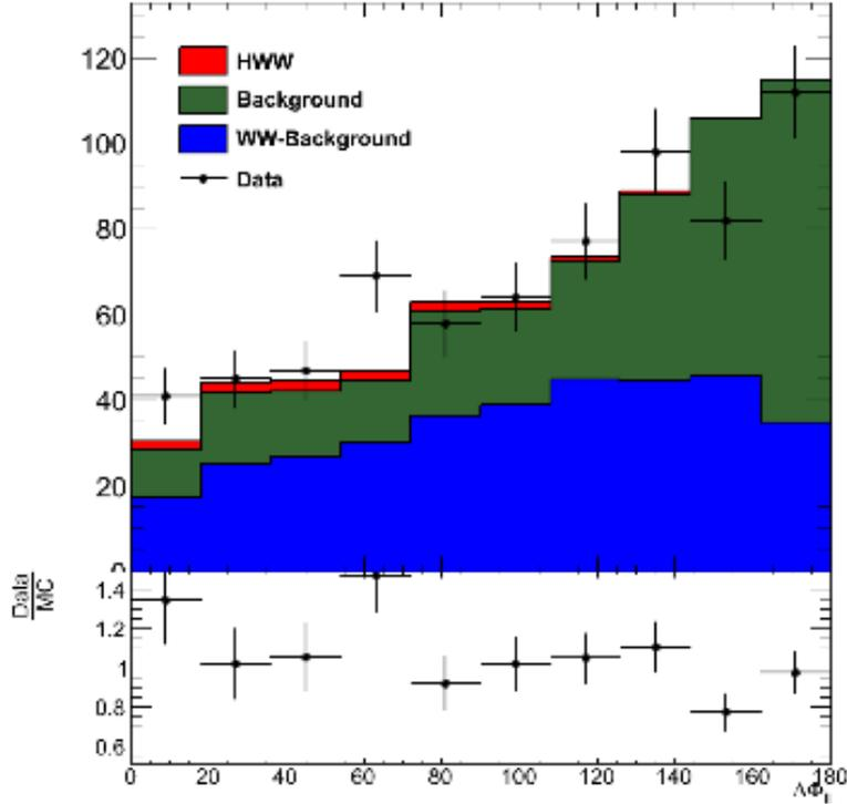
Figure 3: Distribution of the the angle between the two leptons  $\Delta\Phi_{ll}$ . The simulated background is divided into background due to WW pairs not coming from Higgs events and all other background processes.
